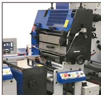
Servo driven flexographic print/coating station
